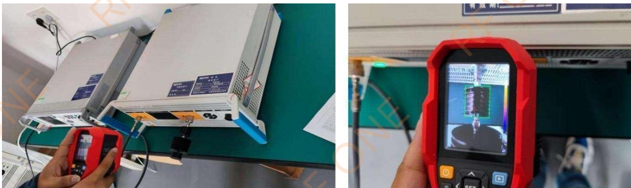
Pic 2 Measure case temperature of DUT
