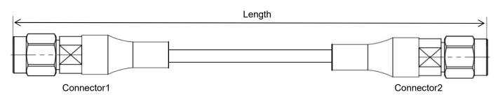
• Length can be in meter or in inch etc, e.g, FL520-SMAM-SMAM-1M. Standard length tolerance: ±1.5%. Custom lengths and other connector types available.
