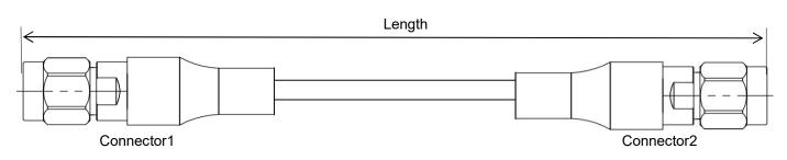
• Length can be in meter or in inch etc, e.g, SP280-292M292M-1M. Standard length tolerance: ±1.5%. Custom lengths and other connector types available.
