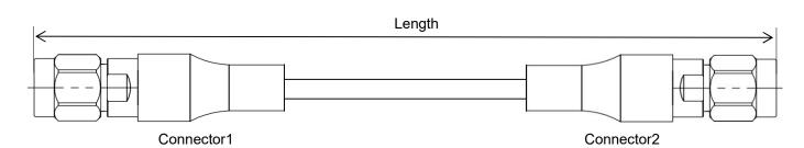
• Length can be in meter or in inch etc, e.g, UF450-292M292M-1M. Standard length tolerance: ±1.5%. Custom lengths and other connector types available.
